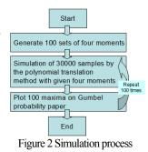
based on the polynomial translation method has been introduced in Choi and Kanda (2003). Figure 2 shows the simulation flowchart. When the simulation process is carried out, the moment method is then applied to obtain the Gumbel parameters from the median estimates of annual maxima and considered as the characteristics of the extreme value distribution.
